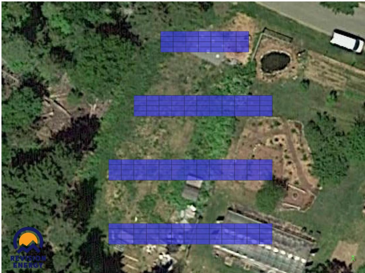
Figure 1: Engineer's rendering of proposed 60.7 kW ground mounted Solar Array.
